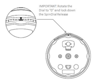
Step 2: Take note of the 3 ports (holes) surrounding the spindle insertion point on the lock cover as pictured below. These "Locator Ports" will be used to position the cam inside the lock correctly for SpinDial access.
