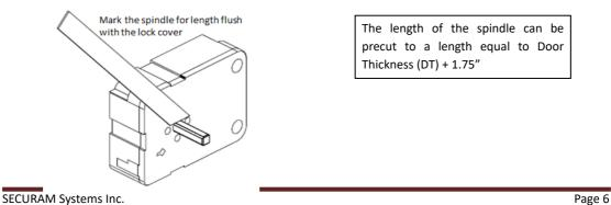
Step 10: Remove the spindle bolt (Part# M4\*16) and spindle (Part# MSP-15A-6IN) from lock case prior to cutting. Carefully cut the spindle so that it will be flush to the lock cover.
