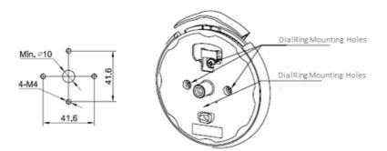
vote: In most safe installations, there are only two plaiking mounting holes, either aligned vertically or horizontally. Two bolts are adequate to secure the DialRing in place.
