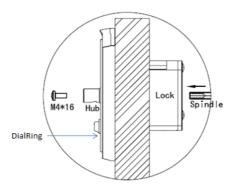
Step 15: IMPORTANT: Now from the Lock body side, tighten the small Phillips head screws to lock the spindle into place at the cam.
