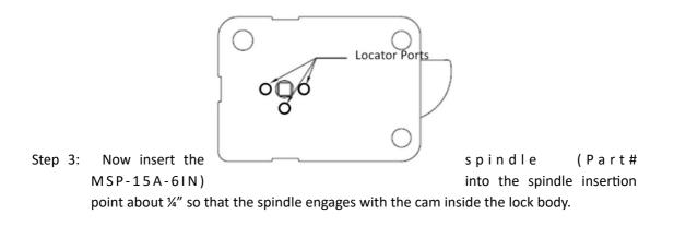
Step 4: Turn the spindle until the three small Phillips head screws are visible in the Locator Ports as shown as demonstrated in picture below.
