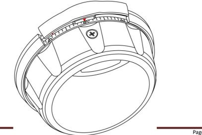
Step 3: Now rotate the SpinDial to the right until it comes to a stop (within one revolution)
